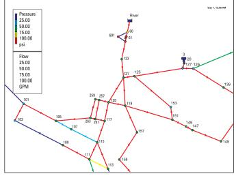
Figure 2-3. EPANET Graphical Output Showing Flow and Pressure.
