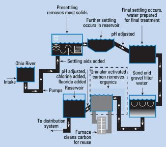
*Figure 1-1. Water Treatment Process at the Miller Plant on the Ohio River (Adapted from: GCWW 2005).*
