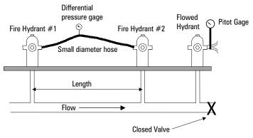
Figure 4-4. Schematic of Parallel Hose C-Factor Test Setup.
