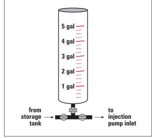
Figure 3-1. Flow Calibration Tube.
